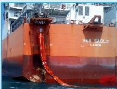
Floating Hose Installation to FPSO
