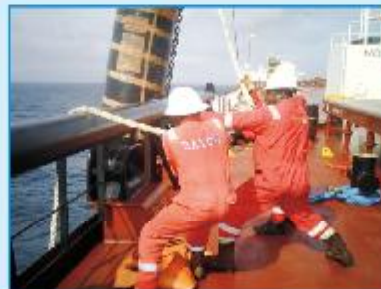
Picking up hose string to connect to tanker export manifold
